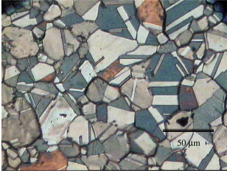
Figure 3. Typical optical image of normal bulk copper prepared in the same method described in section 2.1.1.
